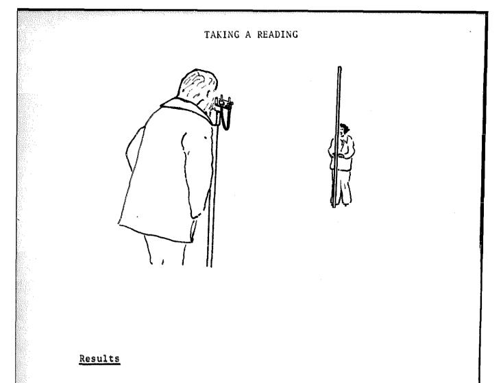
The staff could be read at a distance of 8-10 metres, but this range depends on the operator's eyesight. A 50 metre line was laid out 'on the contour' and checked with a modern optical surveying level. The worst error was 42mm in height over a horizontal distance of 8 metres.
