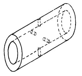
Bush bearing showing the four lubrication holes (full size).
