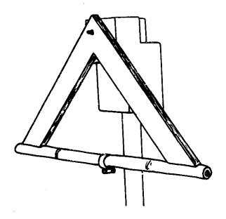
DETAIL OF THE ROAD TRACER SHOWING THE HOSE CLIP ON THE BAMBOO POLE
