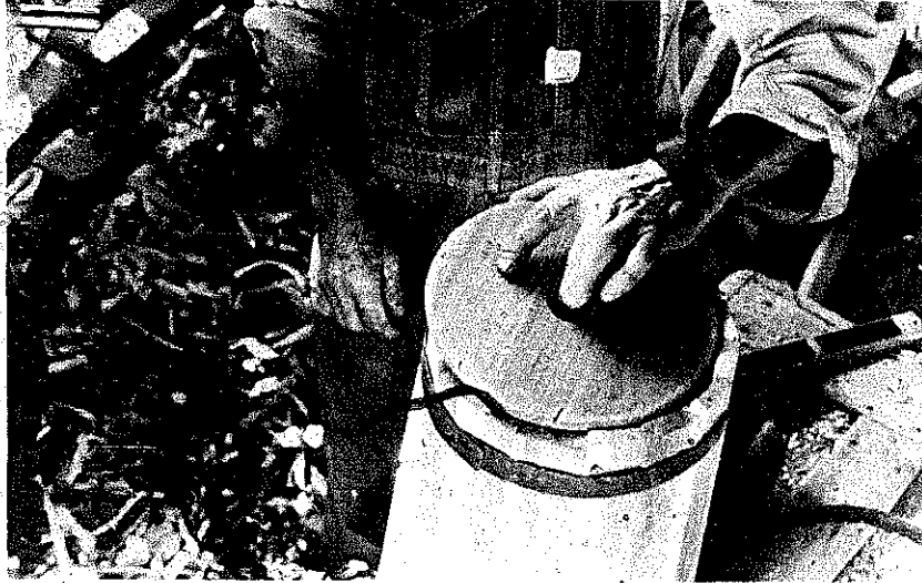
PLATE 390 The top should fit right on top of the churn, with a hole in the middle that the dasher handle can easily slide through.
