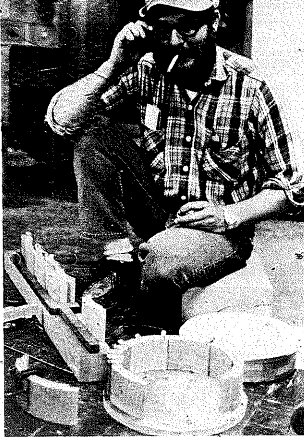
PLATE 127 Dave has his pieces figured out so carefully that he can get every wooden piece he needs out of one 40" x 3" x 3" piece of stock.
