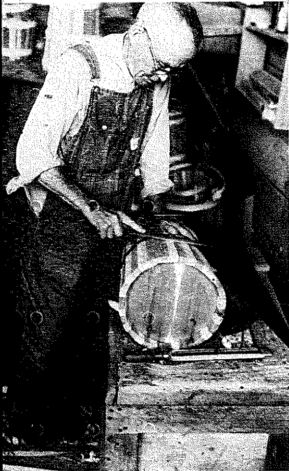
PLATE 370 Step 14: With the temporary bands still on, smooth outside of the churn with a wood rasp.
