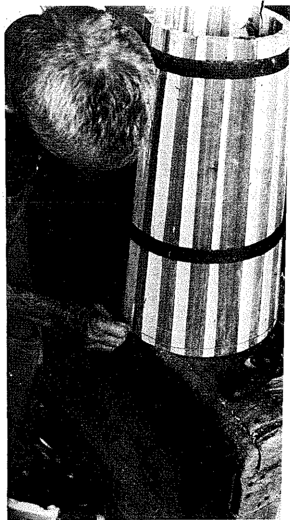
PLATE 371 Step 15: To measure for a permanent bottom hoop, take a string and measure the very bottom of the churn.
