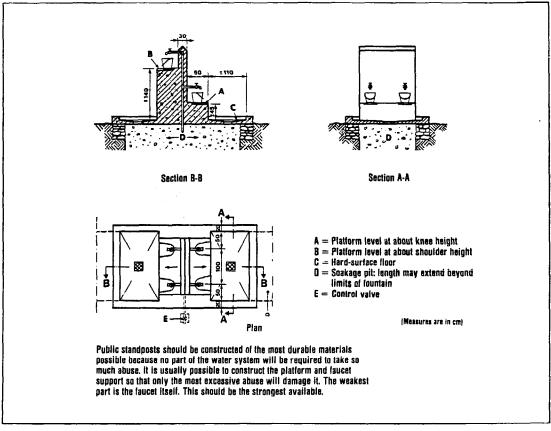
Figure 17. Possible arrangement of public standpost.
