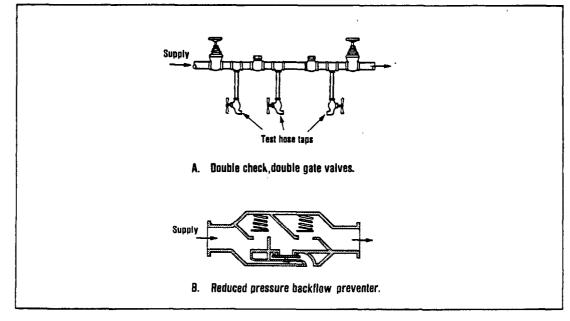
Figure 10. Backflow prevention devices.
