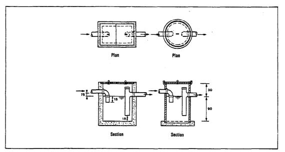
Figure 12. Typical grease traps.
