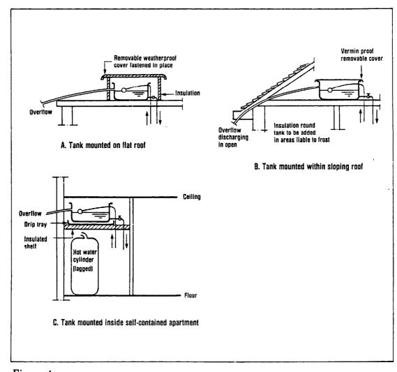
Figure 4. Water storage tanks.
