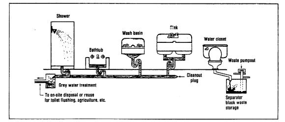
Figure 15. Greywater-blackwater system.
