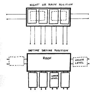
SOLAR HERB DRYER Upper and Lower Trays Slide Out in Three Directions
