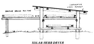
Drying Trays Slide on Rails. One Roof Covers Two Levels of Trays.
