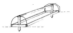
Fig. 6 New Cloche Showing Framework and Kalwall and One of the End Flaps
