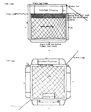
Figure 1. Design of a 64 cubic foot floating fisb cage.
