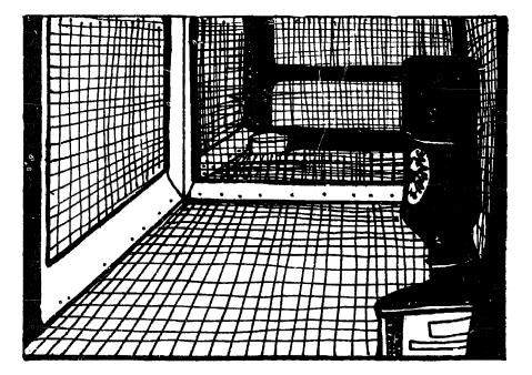
Hutch floors must be "self-cleaning" to prevent disease. No manure will collect in this hutch. Every wood support is covered with sheet metal.
