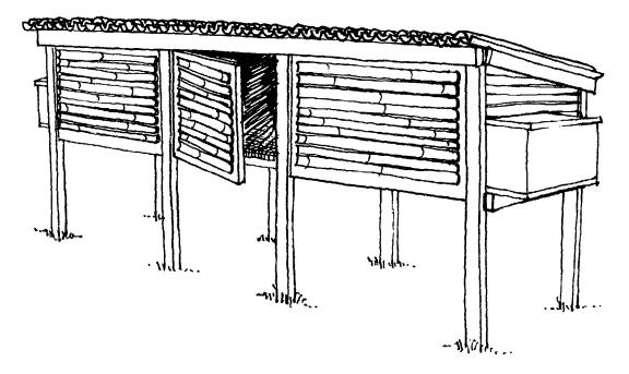
Frame a door to cover the entire front of each cage, and cover with bamboo strips nailed into each frame. Attach the doors to the hutch with two 4" hinges each and a latch for each.
