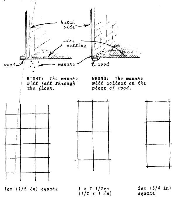
The three most common wire sizes used for flooring. Left, lcm (1/2 in) square, which is good for most projects. Middle, 1 x 2 1/2cm  $(1/2 \times 1 \text{ in})$  "ideal size", usually 16 guage thick. Right, 2cm (3/4 in) wire netting. Somerimes young rabbits' legs are broken by slipping through the holes of this size netting.
