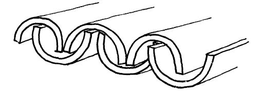
To make a roof, split bamboo lengths into halves, chip out the "nodes" with a hammer, paint the inside surfaces with a waterproofing substance like creosote or solignum, and nail down onto the top of the hutch frame in an interlocking pattern (shown above). Make the bamboo lengths long enough to overlap the front and back of the hutch.
