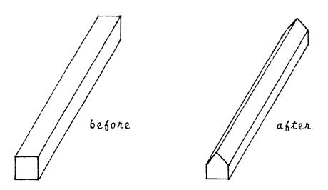
With only an edge supporting the wire, droppings will fall away on each side of the wood and keep the floor clean.
