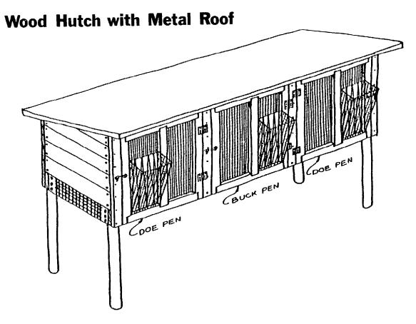
VITA Volunteer George R. Clark has prepared these construction steps from plans provided by Harlan Attfield. Some construction tips: Be sure all edges on floor are flush, so all rabbit droppings fall to the ground.
