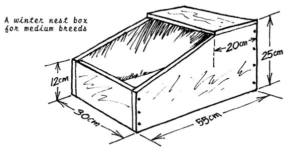
This closed-top winter nest box will hold the body warmth of the baby rabbits. These nest boxes can be made of 1cm (1/2") or even 2 1/2cm (1") lumber. One 4 x 8' (about 1.2 x 2.4m) sheet of plywood will make four of these boxes, with just a little left over. Use wood for these boxes. If metal is used the box will "sweat" and create a health problem for the young rabbits.
