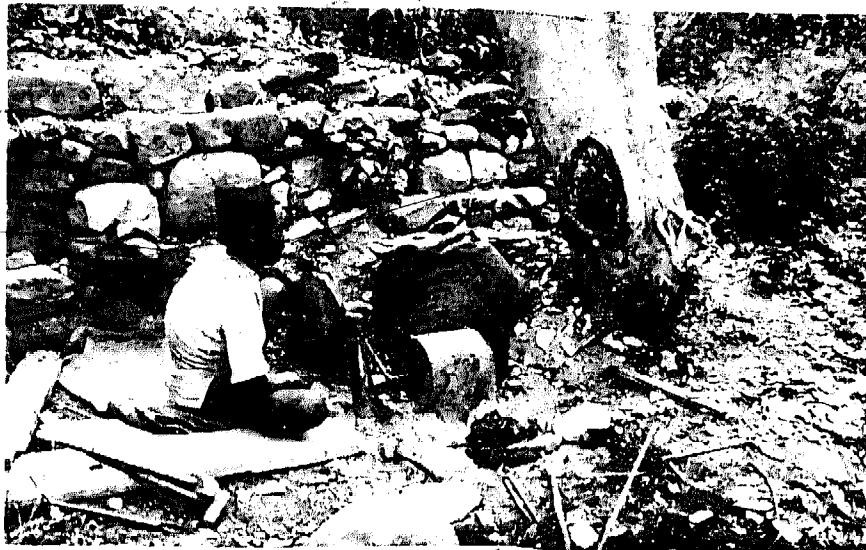
A blacksmith's field workshop. The smith blows air in to the charcoal fire.
