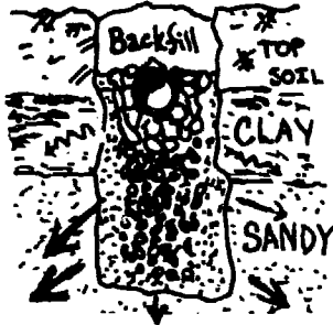
Top: a poorly placed trench with sidewalls in clay layer.
