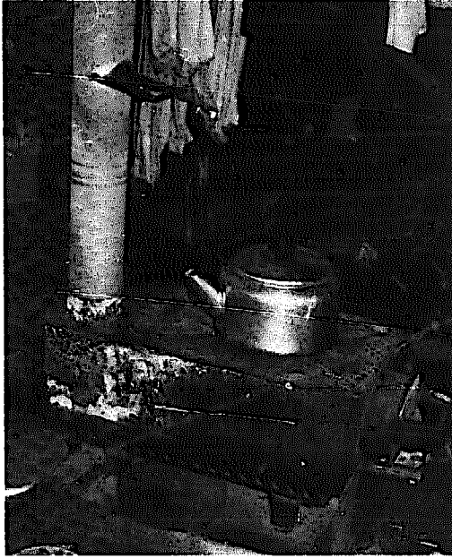
Figure 16.15—Squared one-third-barrel stove. Note tin-can damper in pipe, and small area of pipe retaining original galvanized luster just above the damper slit. Made by Oliver Cameron.
