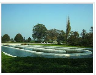
Raceway pond used to cultivate microalgae. The water is kept in constant motion with a powered paddle wheel.
