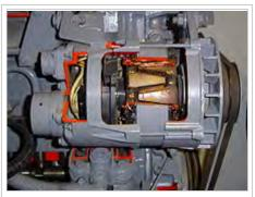
Cut-away of an alternator, showing the claw-pole construction; two of the wedge-shaped field poles, alternating N and S, are visible in the centre and the stationary armature winding is visible at the top and bottom of the opening. The belt and pulley at the right hand end drives the alternator.
