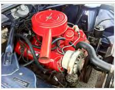
Alternator (silver) mounted on a V8 engine
