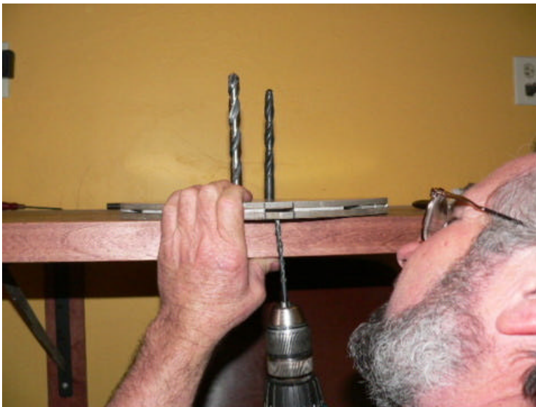
(drilling into the bottom magnet rotor)
