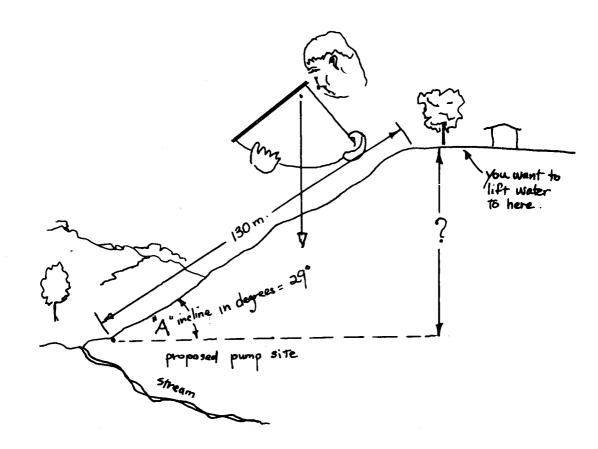
Compute the height, using a table "Natural Values of Trigonometric Functions". From trigonometry we have the following formula:
