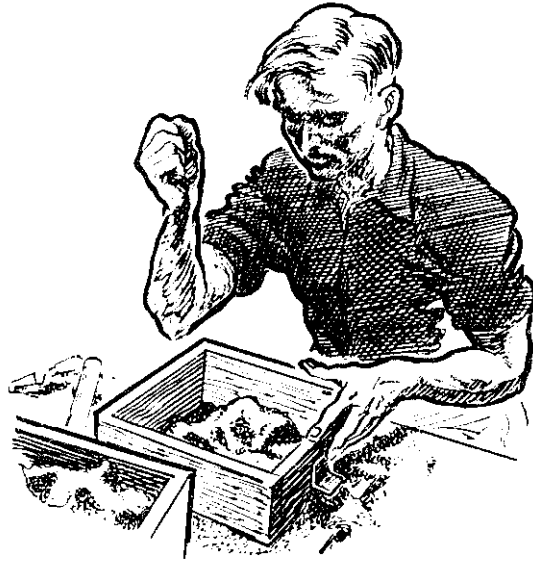
Fig. 57. Moulding by sand slinging.
