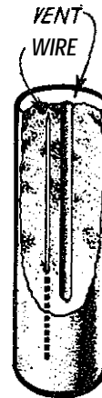
Fig. 46. Showing how a sand core can be vented and also reinforced with wire.
