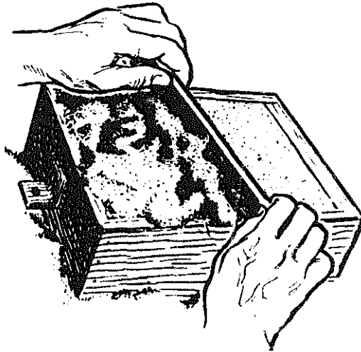
Fig. 59. Strickling away the surplus sand.
