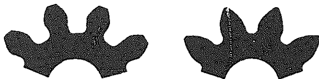
Figure 4. Left, a 10-tooth pinion with undercut resulting from pressure angle of 14\frac{1}{2}^\circ ; right, without undercut because of a larger pressure angle.
