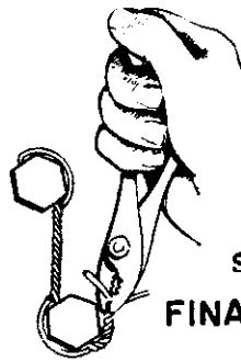
Figure 32. Standard twist safety wire installation procedure.
