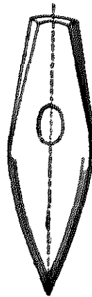
Fig. 67—Showing how the Hammer Marks are Ground out.
