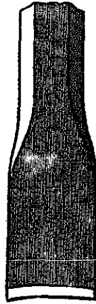
Fig. 48—Improperly Ground Chisel.
