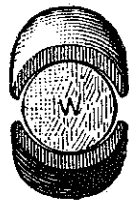
FIG. 142.—SHAPE OF TONG JAWS FOR ROUND WORK.
