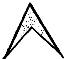
Fig. 385—Showing the Steel After it has been Cut into and Doub'ed Around.
