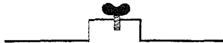
FIG. 198.—SHAPE OF SIDE IRONS HOLDING THE AXLE OF FAN IN "NO NAME'S" BLOWER.
