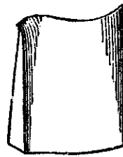
FIG. 82.—SHAPE OF METAL WEDGE.
