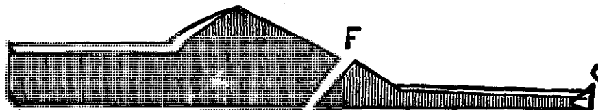
Fig. 369—Showing how the Two Pieces are Welded.
