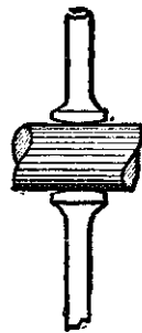
Fig. 200—Right way to Shape Calliper Ends. Fig. 201—Wrong way to Shape Calliper Ends.
