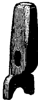
Fig. 2—Collaring Tool for Shouldering Down Round Iron. Made of 1\frac{1}{4} square Steel.
