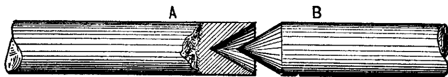
Fig. 105—Welding a Round Shaft, by the Method of “H. H. L.”
