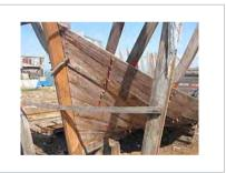
Plank fixing, trenails and red lead paint, Quy Nhon.
