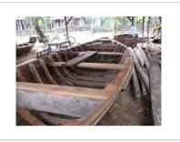
Boat nearing completion with frames added. Hoi An.
