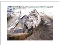
Small boat using the planks first method. Hoi An.
