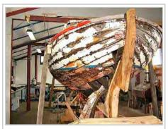
Damaged boat mid-reconstruction; carvel planking partially removed.
