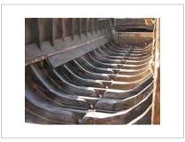
Repaired frames, barge hull. Sa Dec, Mekong Delta.
