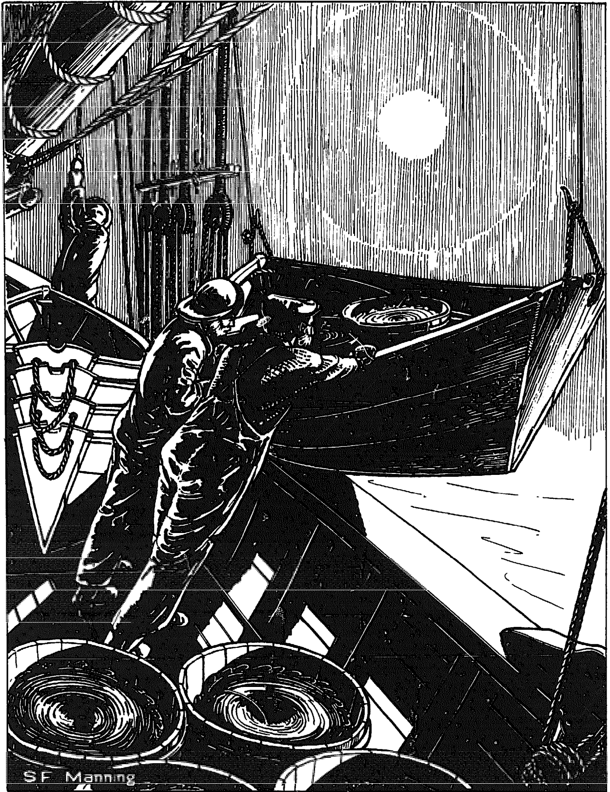
In a fishing schooner, the dories were hoisted in and out by tackles made up to the crosstrees of the schooner's masts. A hooked rod, or dory book, at the end of the dory tackle permitted over-the-rail fishing for the rope buckets of a dory alongside.
