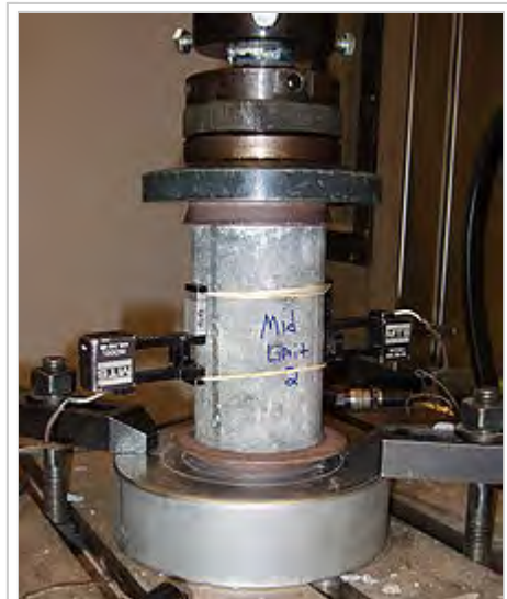
Compression testing of a concrete cylinder. Photo courtesy of Simpson Gumpertz & Heger, Inc.
