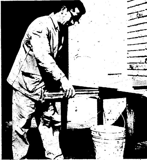
Fig. 20 Testing the tensile strength of a soil-cement block.
