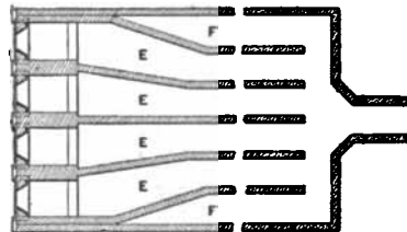
FIG. 12.—SETTING OF SALT-PANS.
