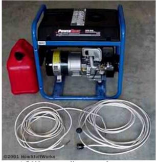
A 5,000-watt gasoline-powered generator This generator has a 10-horsepower engine and a 5,000watt generator with a surge rating of 6,500 watts. The gas tank (black, mounted across the top of the frame) holds 7 gallons and runs about 12 hours at 1,000-watt usage levels. This generator produces 120-volt or 240-volt output. It is shown with its grounding cable and the 240-volt cable that plugs it into the house's circuit panel.
