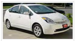
This 2004 Toyota Prius hybrid has an Atkinson cycle engine as the petrolelectric hybrid engine
