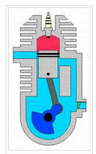
Diagram of a crankcase scavenged 2-stroke engine in operation
