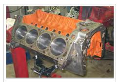
Bare cylinder block of a V8 engine
