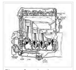
Diagram of an engine using pressurized lubrication
