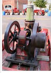
One-cylinder gasoline engine, c. 1910
