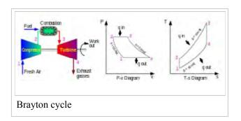
Gas turbine cycle engines employ a continuous combustion system where compression, combustion, and expansion occur simultaneously at different places in the engine—giving continuous power. Notably, the combustion takes place at constant pressure, rather than with the Otto cycle, constant volume.
