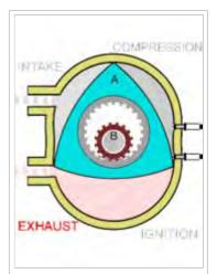
The Wankel rotary cycle. The shaft turns three times for each rotation of the rotor around the lobe and once for each orbital revolution around the eccentric shaft.
