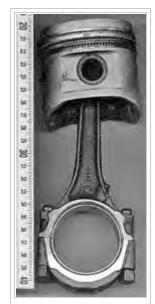
Piston, piston ring, gudgeon pin and connecting rod
