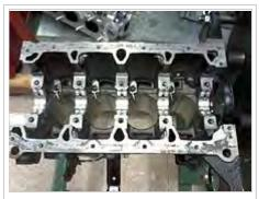
Engine block seen from below. The cylinders, oil spray nozzle and half of the main bearings are clearly visible.
