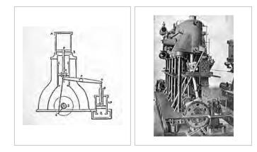
Diagram of a simple "hammer" engine
