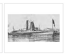
The 1836 paddle steamer *New York*. Between the paddlewheels is the tall square or "A-frame" engine, within which can be seen the long piston rod, near the top of its stroke, making a "T" with the horizontal crosshead
