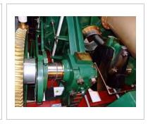
Looking down at the trunk engine of HMS *Warrior* (1860). The connecting rod can be seen emerging from the trunk at right.
