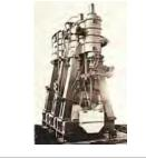
Animation of a typical vertical triple-expansion engine
