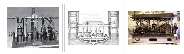
Model of a Maudslay oscillating engine
