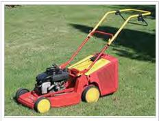
Rotary lawn mower, with a vertical shaft engine
