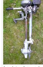
Lateral view of a two-stroke Forty series British Seagull outboard engine, the serial number dates it to 1954/1955
