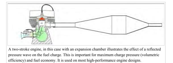
Although the principles remain the same, the mechanical details of various two-stroke engines differ depending on the type. The design types vary according to the method of introducing the charge to the cylinder, the method of scavenging the cylinder (exchanging burnt exhaust for fresh mixture) and the method of exhausting the cylinder.
