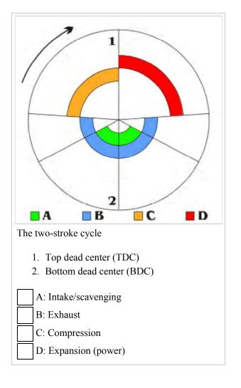
An additional benefit of loop scavenging was the piston could be made nearly flat or slightly dome shaped, which allowed the piston to be appreciably lighter and stronger, and consequently to tolerate higher engine speeds. The "flat top" piston also has better thermal properties and is less prone to uneven heating, expansion, piston seizures, dimensional changes and compression losses.
