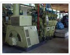
Brons two-stroke V8 Diesel engine driving a N.V. Heemaf generator.
