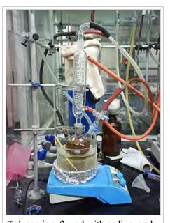
Toluene is refluxed with sodium and benzophenone to produce dry, oxygen-free toluene. The toluene is dry and oxygen free when the intense blue coloration from the benzophenone ketyl radical is observed.
