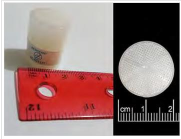
Canisters are commonly filled with silica gel and other molecular sieves used as desiccant in drug containers to keep contents dry.
