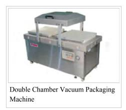
Double chamber sealers require the entire product to be placed in a plastic bag within the machine. Once the product is placed in the machine on the seal bar, the lid is closed and air is removed. Then a seal bar inside the chamber seals the product in the bag, after sealing the bag the chamber is refilled with air
