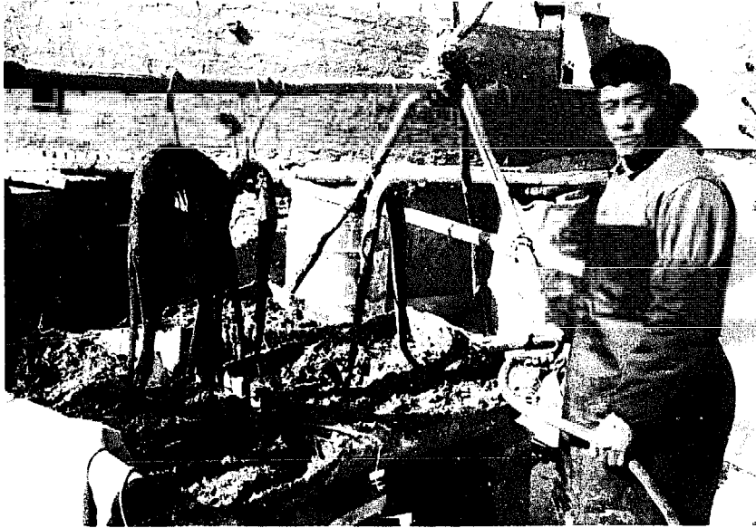
Photo 24 - Mud in half oil drum. Water being added to adjust consistency. Clay/straw bundles hanging above drum. (Niou Pao Tun Depot)
