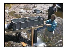
The LH1000 is an exciting hydro turbine that produces DC electrical power at sites with sufficient water flowing across relatively level terrain. The LH1000 uses a durable, low-head bronze propeller to produce power on a head of 2 to 10 feet. At 10 ft of head, the output from this turbine is <u>one kilowatt</u>, which is enough to supply the electrical requirements for an average household.
