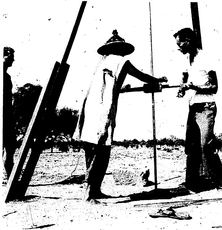
Fig. 11 Drilling with a helical auger
