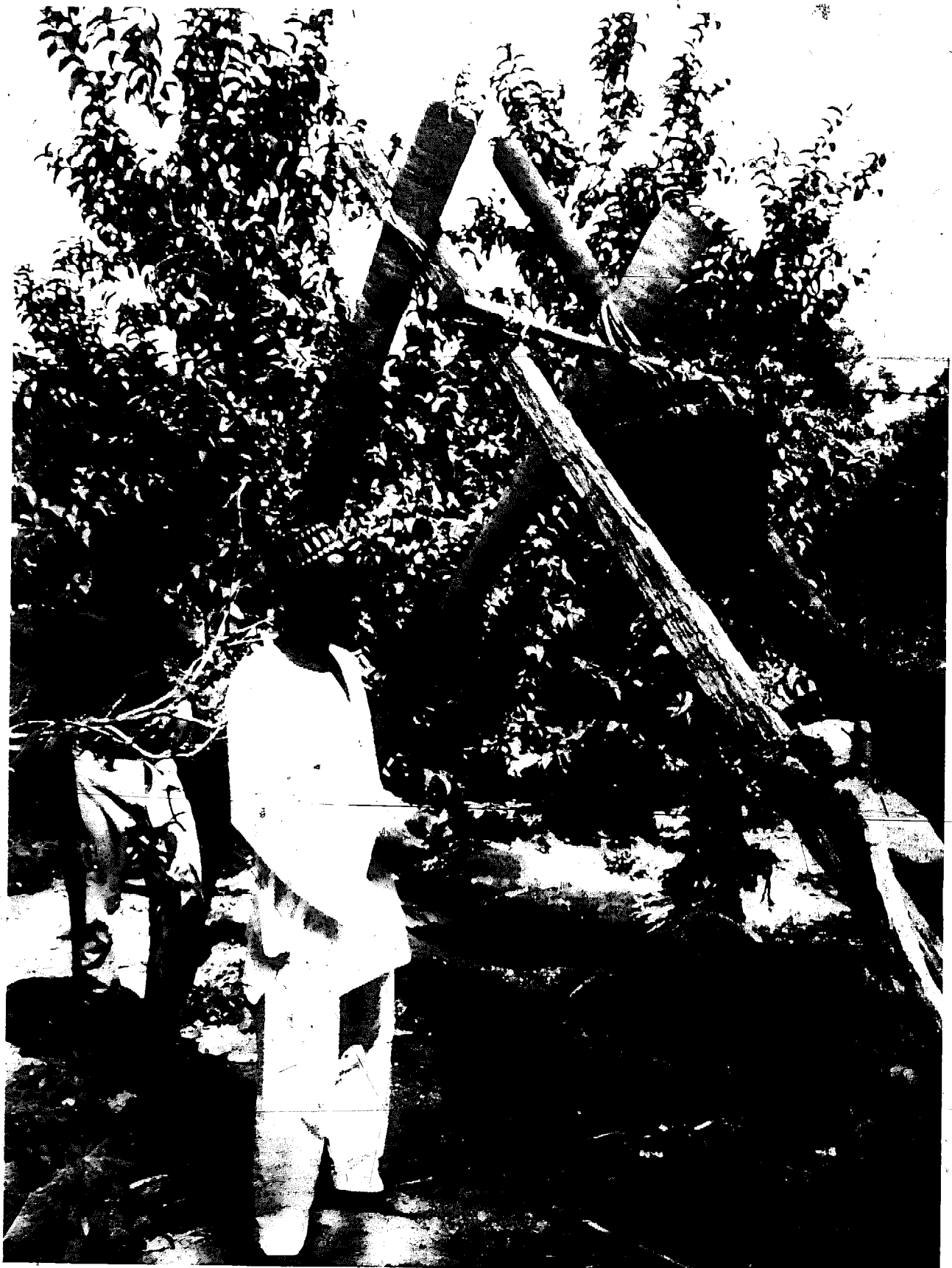
Traditional animal-drawn, skin bucket on large diameter well used in irrigating orchard
