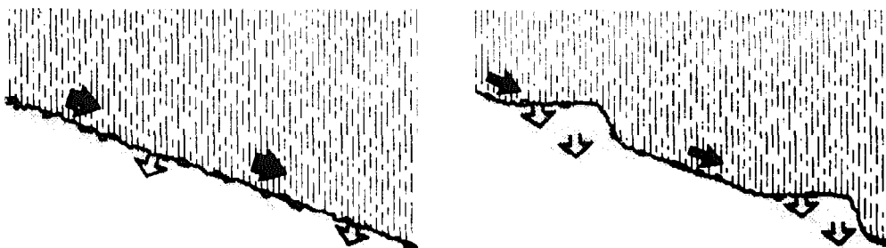
Fig.8 Run-off interception with ridges
