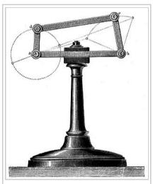
Illustration of a four-bar linkage from Kinematics of Machinery, 1876
