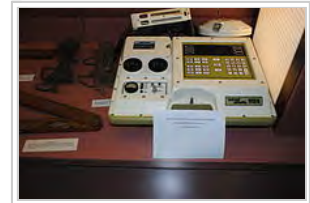
The first portable GPS unit, Leica WM 101 displayed at the Irish National Science Museum at Maynooth.
