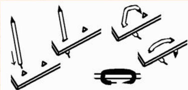
BASIC STEPS INSERTING A QUILL THROUGH BARK
