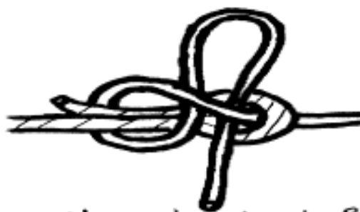
Slipped Sheet Bend
