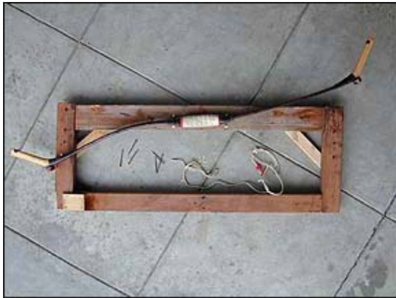
The bow in the stringing jig, with one limb bent.
