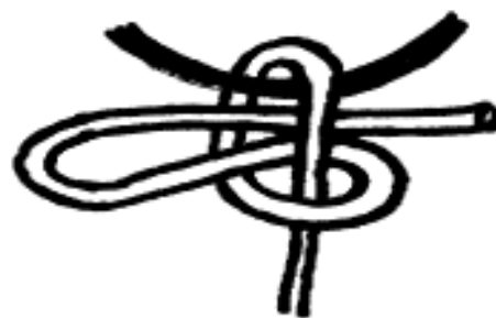
Slipped half hitch
