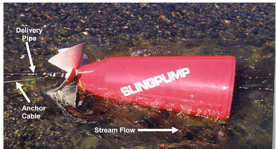
Figure 2 Sling Pump Operating in a Stream
