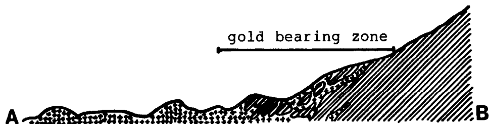
Fig. 2 Map and section with gold bearing contact zone between volcanic and dioritic rocks (According to Brinck, 1955)
