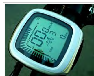
Hybrid bicycle speedometer with integrated battery level measurement.
