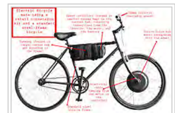
Diagram illustrating a standard bicycle converted to an e-bike using a retail conversion kit
