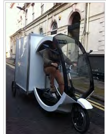
A modern electric cargo trike in use in London, with a payload of up to 250kg
