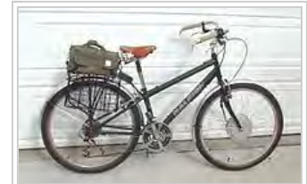
A bike equipped with an after market electric hub motor conversion kit, with the battery pack placed on the rear carrier rack
