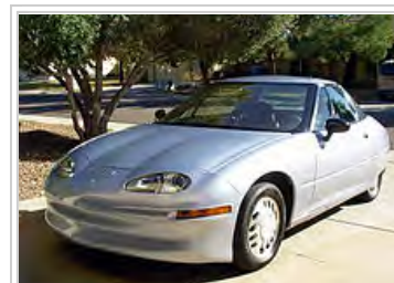
The General Motors EV1, one of the cars introduced due to the California Air Resources Board mandate, had a range of 160 mi (260 km) with NiMH batteries in 1999.
