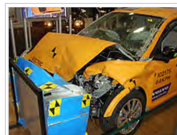
Frontal crash test of a Volvo C30 DRIVE Electric to assess the safety of the battery pack
