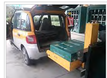
The battery swap process on a Zotye M300 EV.
