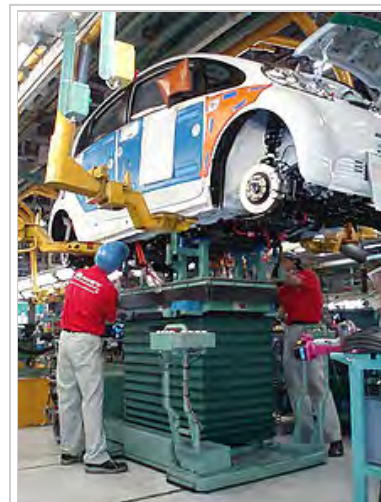
A Mitsubishi i-MiEV having its batteries installed
