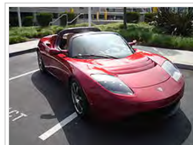
The Tesla Roadster, which began shipping to customers in 2008, uses Li-Ion batteries to achieve up to 244 miles (393 km) per charge while also capable of going from 0 to 60 miles per hour (0 to 97 km/h) in under 4 seconds.
