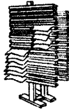
FIGURE 5. A SIMPLE DRYING RACK CAN BE MADE FROM 5 CM. X 5 CM. UPRIGHTS WITH 2.5 CM. X 3.5 CM. CROSSBARS ABOUT 2.5 CM. APART.
