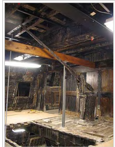
The still-intact aft bilge pump of the Swedish 17th century warship Vasa as seen from the upper gun deck.
