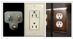
NEMA 5-15 plug, left. Decorative-style duplex socket, with orientation as specified in NECA 130-2010, center. Ordinary duplex socket, with orientation typically found, right. Photos are different scale-parallel blades are on 1/2 inch (12.7 mm) centers.
