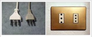
Side by side comparison of Italian CEI 23-50 S 11 and S 17 plugs and sockets rated 16 A (left) and 10 A (right). Italian plugs and sockets are defined by the standard CEI 23-50 which superseded CEI 23-16. This includes models rated at 10 A and 16 A that differ in contact diameter and spacing (see below for details). Both are symmetrical, allowing the line and neutral contacts to be inserted in either direction. This plug is also commonly used in Chile and Uruguay.
