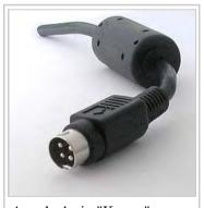
A male 4-pin "Kycon" power connector, which appears similar to a Mini-DIN connector
