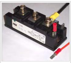
High-power transistor switch module with large screw connectors and small crimped-on "Fast-on" connectors
