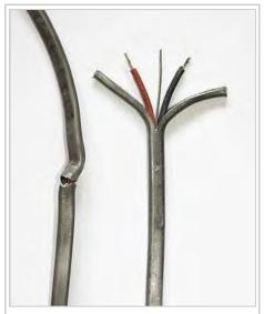
Lead cased electrical wire from a circa 1912 house in Southern England. Two conductors are sheathed in red and black rubber, the central earth wire is bare. These wires are dangerous because the sheath is prone to split if repeatedly flexed.
