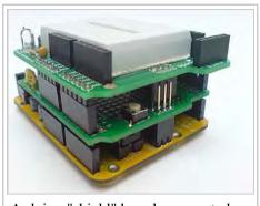
Arduino "shield" boards connected via stackable bus connectors
