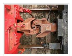
Paired "knuckle" type hermaphroditic mechanical couplers for railcars (viewed from above)
