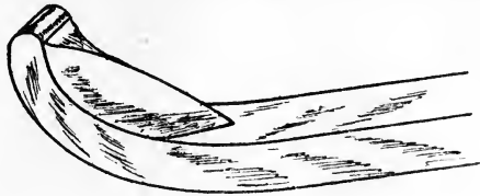
FIG. 91.—Streamlining curved toe of skid.
