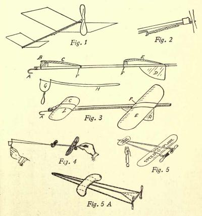
with a forward and rear plane of cardboard or onion-paper. The propeller may be cut from thin sheet celluloid, aluminum, or stiff cardboard, and is turned by a twisted rubber
