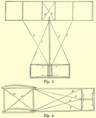
Each section, except the small central ones, should be thus wired; but as the diagonal crossed wires would interfere with the operator in the central section, another method is carried out in this.
