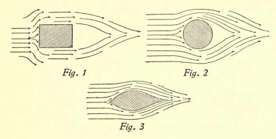
body form," and is the sectional shape of most of the spars, struts, beams, and other parts of the modern aeroplane.
