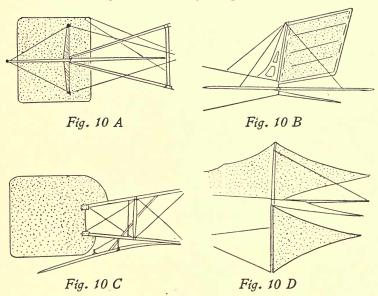
fabric and usually placed in the rear of the machine on the tail, with about half of its surface above and half below the horizontal tail and elevators. Fig. 10 A shows the rudder on the tail of a Curtiss biplane, Fig. 10 B the rudder on the tail of a Benoist, Fig. 10 C that of a Bleriot monoplane, and Fig. 10 D the rudder and elevator of an Antoinette.
