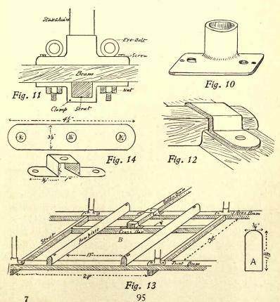
Screw each socket in place with small wood-screws with round heads through the smaller holes in the base.
