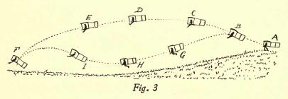
At A the flier is just starting to run forward on the hilltop, and the line from A to B shows how his flight or glide starts at first.
