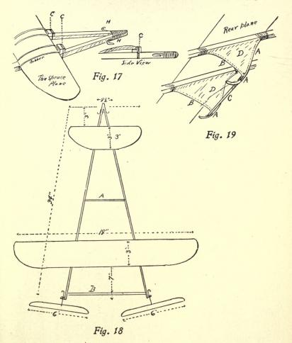
The braces are lashed and glued to the skids, and both skids and braces are lashed to the frame, with the upper end of the braces four inches from the rear end of the beams, and the front upper ends of the skids seven inches from the rear, or, in other words, 2-1/2" from the ends of the braces (Fig. 19, A, B).
