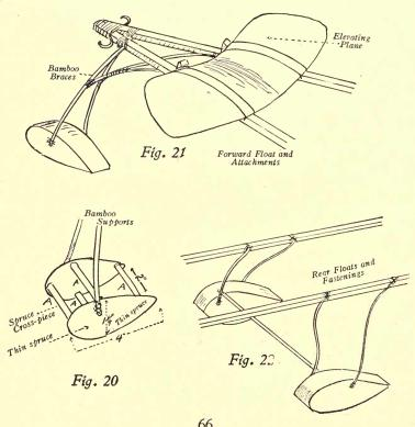
The forward pontoon is 4" long and 2" wide and 1-1/4" deep, constructed by cutting two pieces for the sides (Fig. 20), separated by four braces, as shown in Fig. 19, A, A, each 3/16" square.
