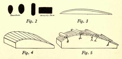
in position while drying by cleats placed across them and held down to the sides of the form by a hook or by twisted wire, as shown in Fig. 5.
